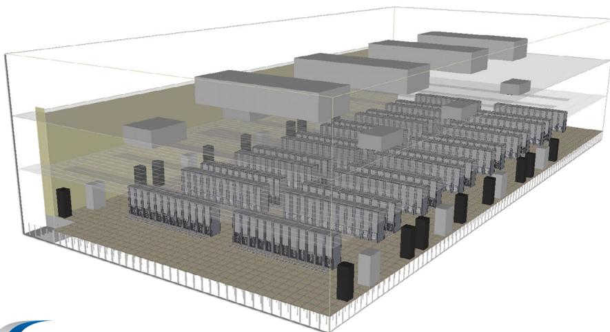
*(Left) The Shakopee, MN, data center as modeled in the Virtual Facility. The facility has 13,000 ft<sup>2</sup> raised floor space with no columns; a 12 ft drop ceiling used as a return air plenum; a 36" raised floor; 1.2 MW of critical IT load; four roof top air handlers in an N+1 configuration; and 336 25%-open perforated tiles with dampers installed.*
